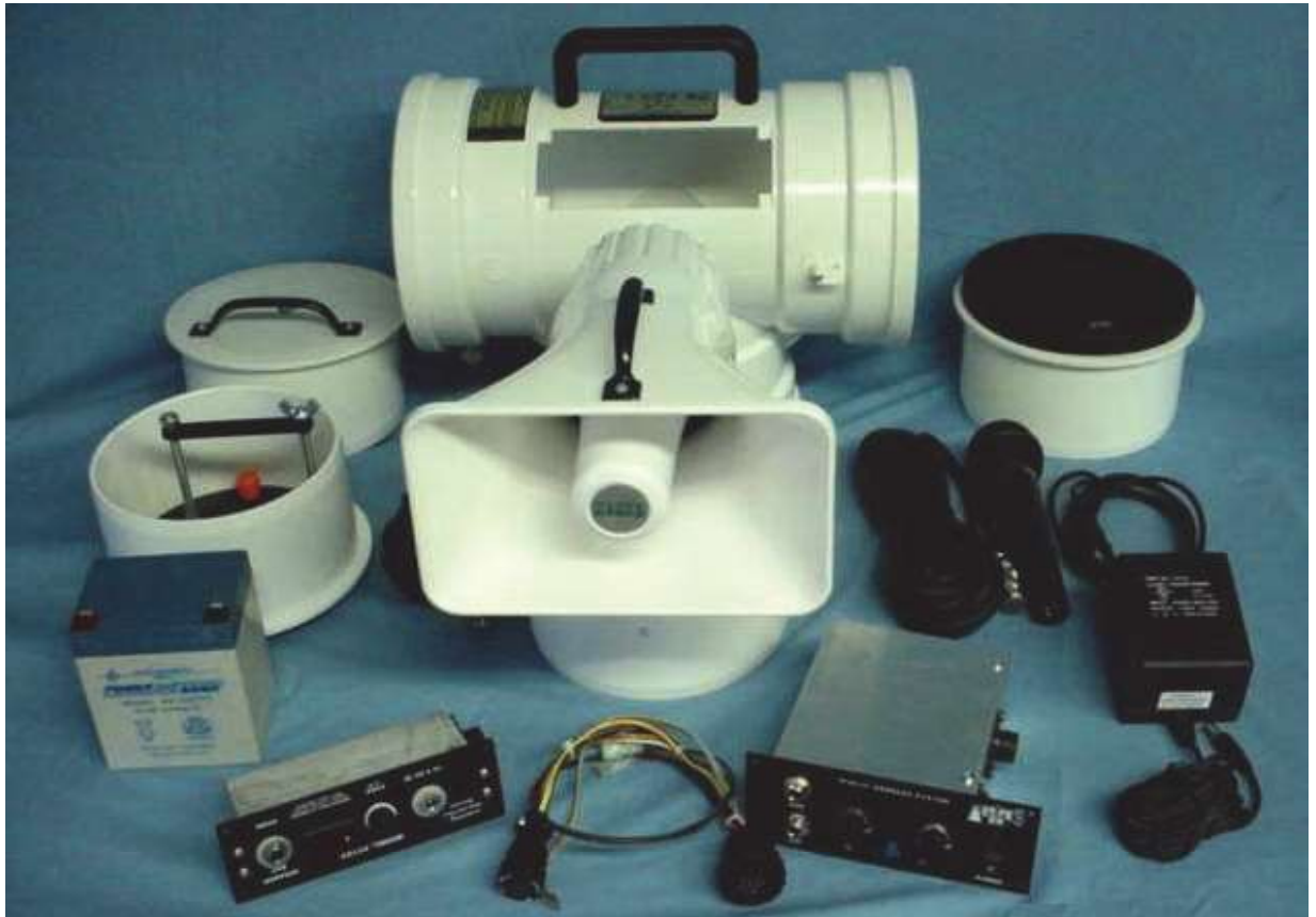
FIGURE 1 COMPONENTS OF POWER T
