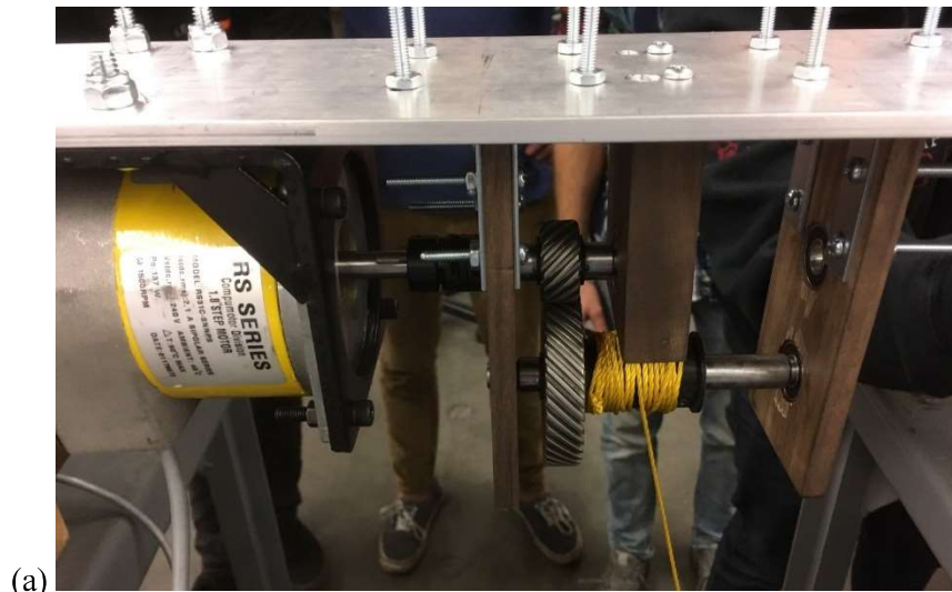
FIGURE 6 ELECTRIC CEILING HOIST FROM GROUP 3; (A) TESTING, (B) ASSEMBLY
