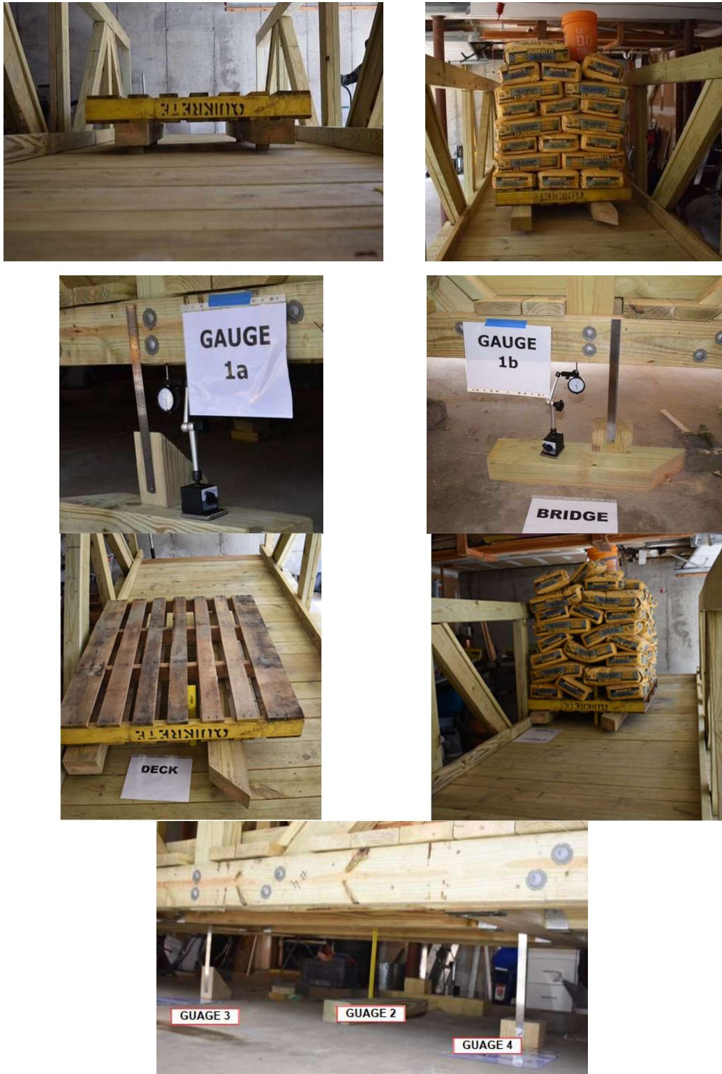
FIGURE 2 DEFLECTION TEST PHOTOS
