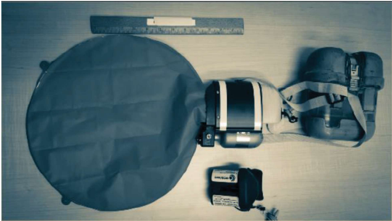
FIGURE 1 (TOP) A 10-MINUTE DURATION SCSR UNIT (LEFT) AND CARRYING CASE (RIGHT); (BOTTOM) SCSR SIMULATOR EXPECTANCY TRAINING DEVICE. A 12-INCH RULER IS PROVIDED FOR SCALE
