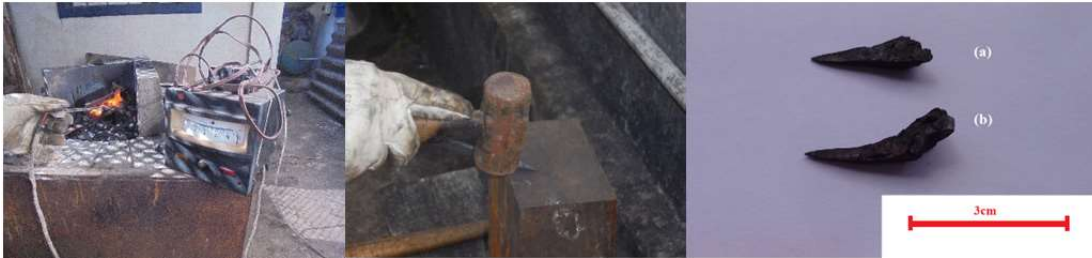
FIGURE 2 DETAILS OF THE WHOLE PROCESS TO OBTAIN THE ARROWHEADS: (A) THE FORGE (FIRE, THERMOCOUPLE, FRAGMENTS BEING HEATED); (B) HAMMERING; (C) ARROWHEADS A (AIR COOLED) AND B (QUENCHED)
